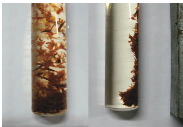
Figure 8 Paragraphs of magnetic \gamma -Fe 2 O 3 /chitosan composite films dispersed in dye solution (left) and the response to a magnetic field (right). [Color figure can be viewed in the online issue, which is available at wileyonlinelibrary.com ].
